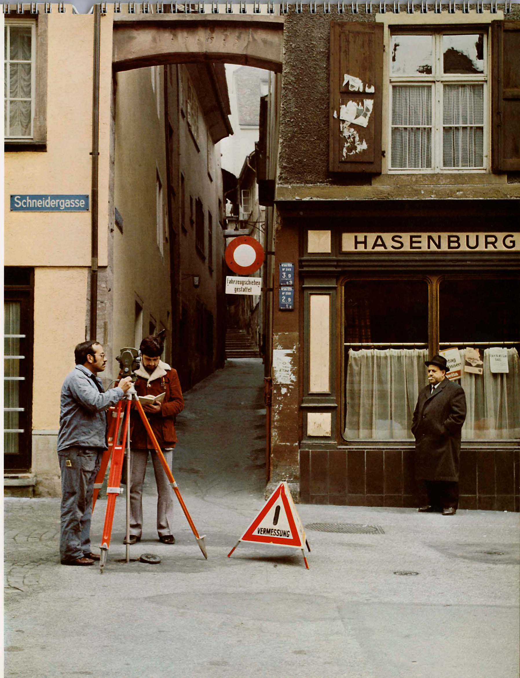
The Kern DKM2-A one-second theodolite with attached Kern DM 500 electro-optical distance meter during detailed survey in the old city of Basel
