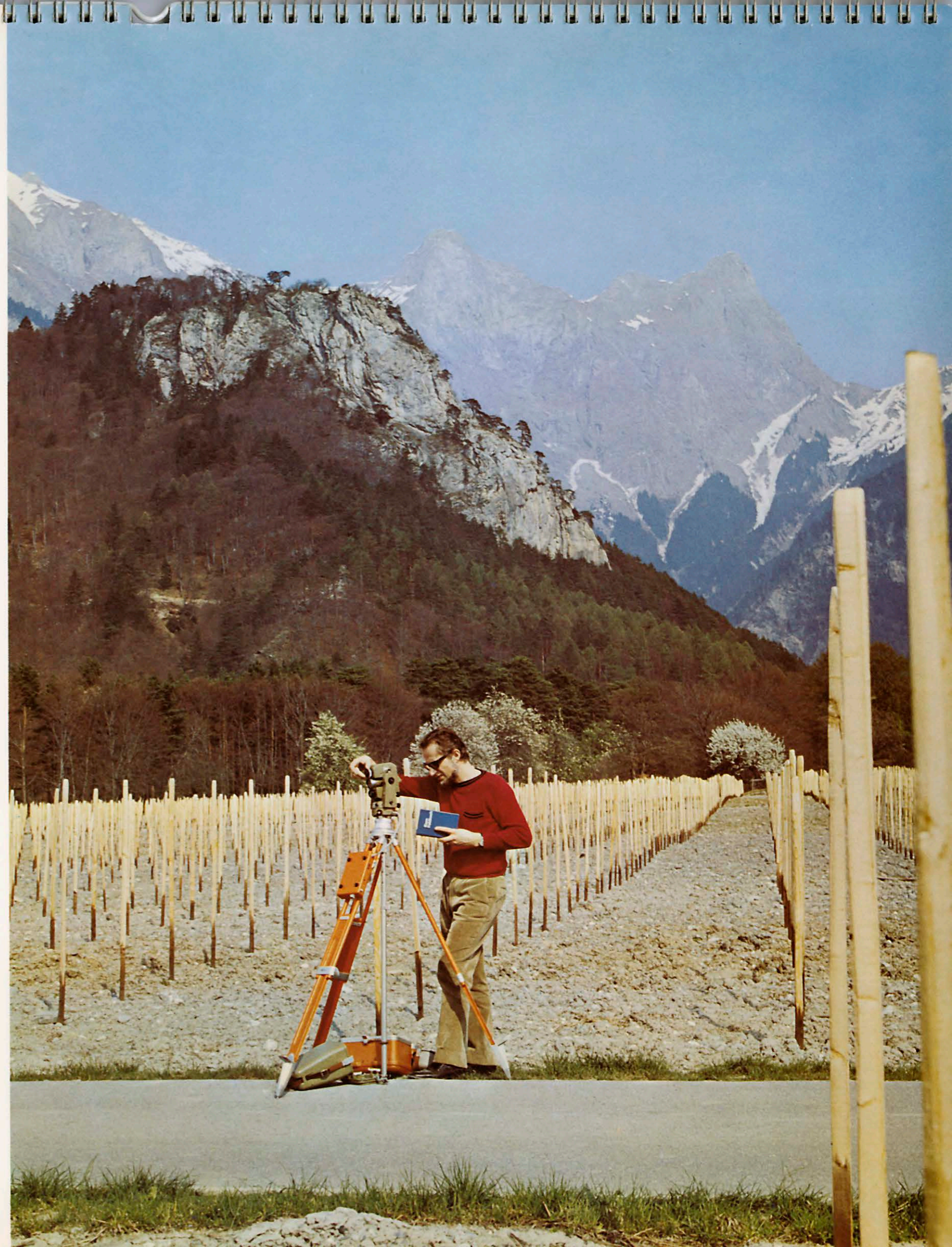
Cadastral survey in a vineyard at Fläsch (Grisons) with the Kern K1-S engineer's theodolite combined with the Kern DM 500 electro-optical distance meter
