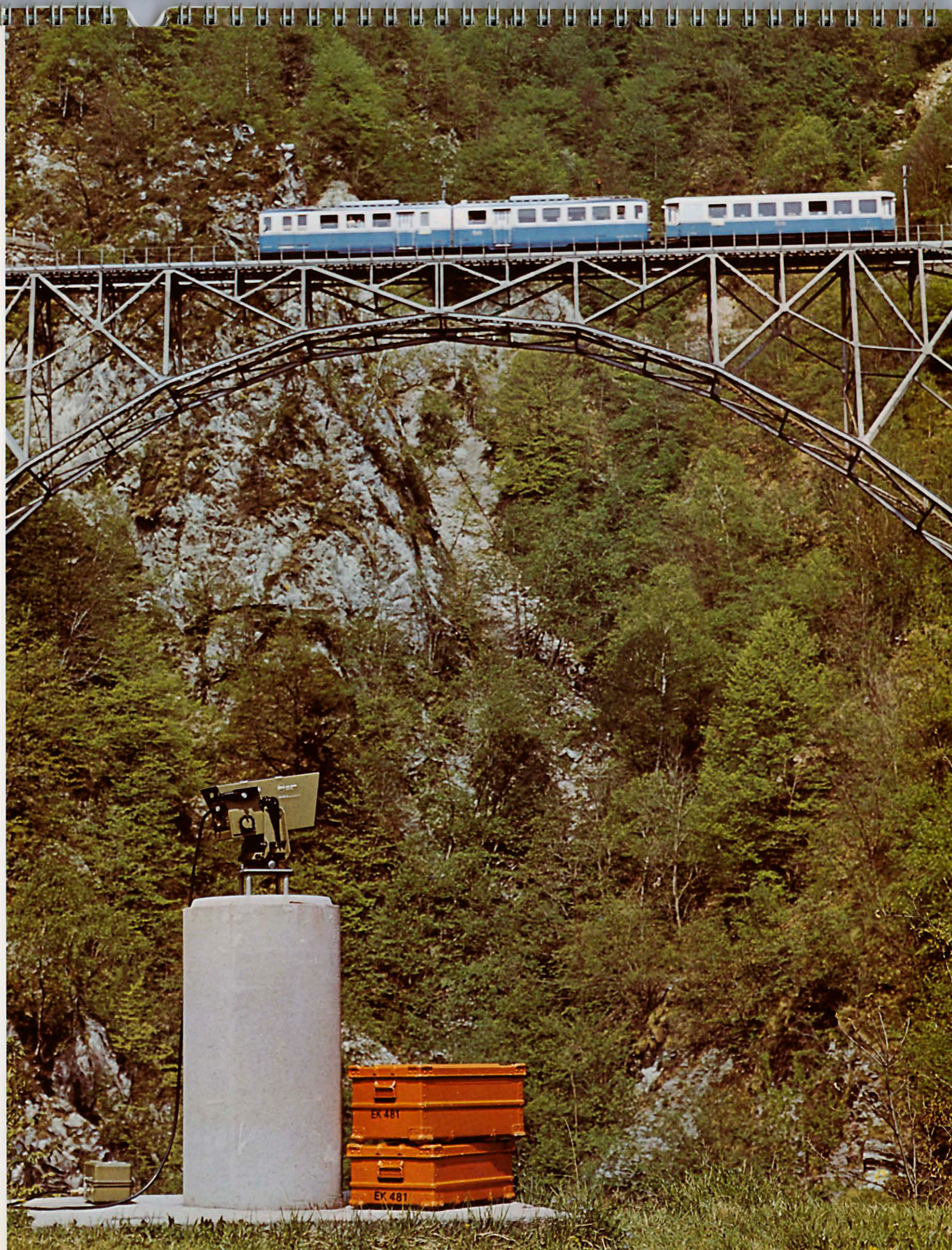
Control measurement on a railway bridge at Camedo (Centovalli, Ticino), carried out with the Kern ME 3000 Mekometer
