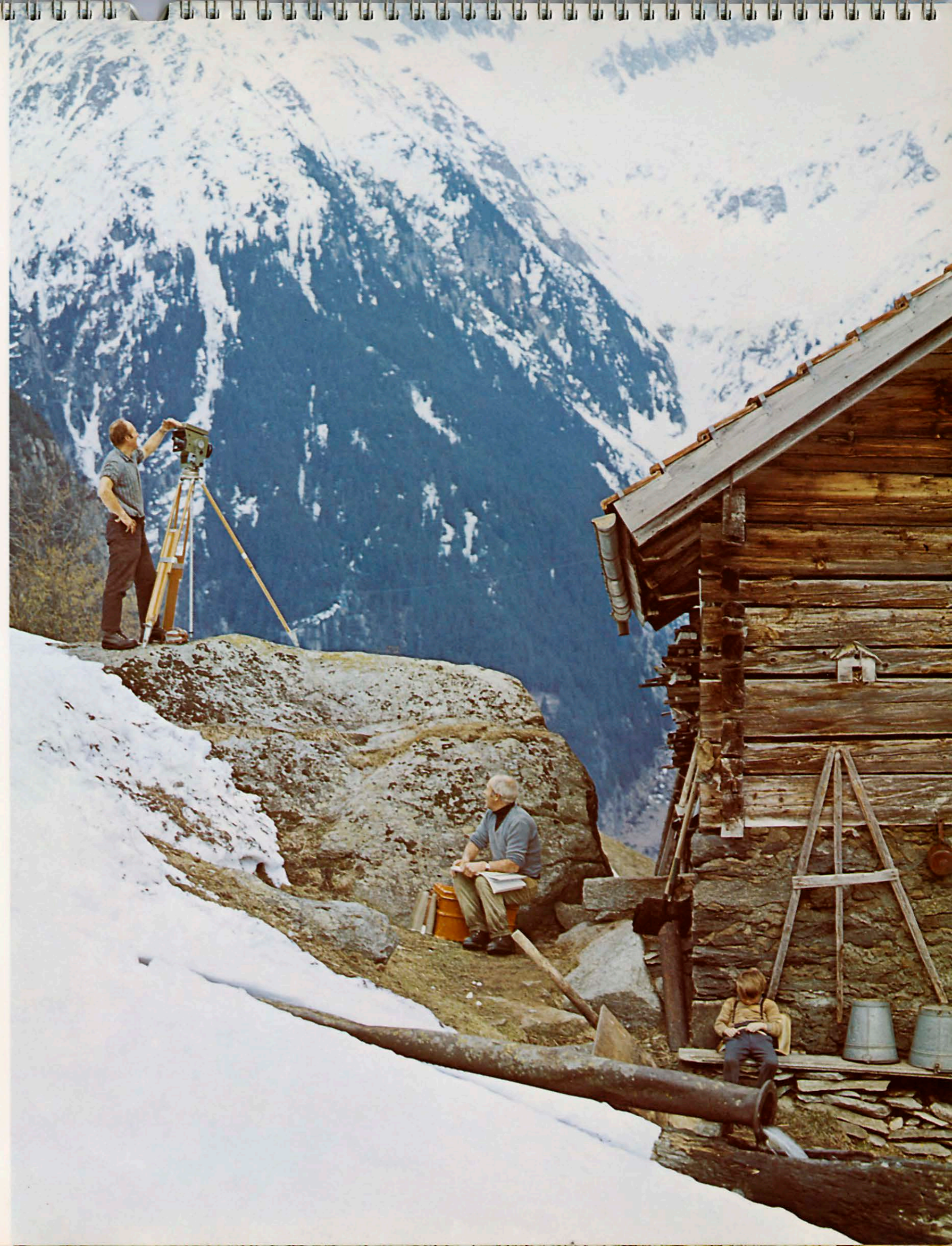
Densification of a fixed point network at Göschenen (Uri) with the electro-optical distance meter Kern DM 2000
